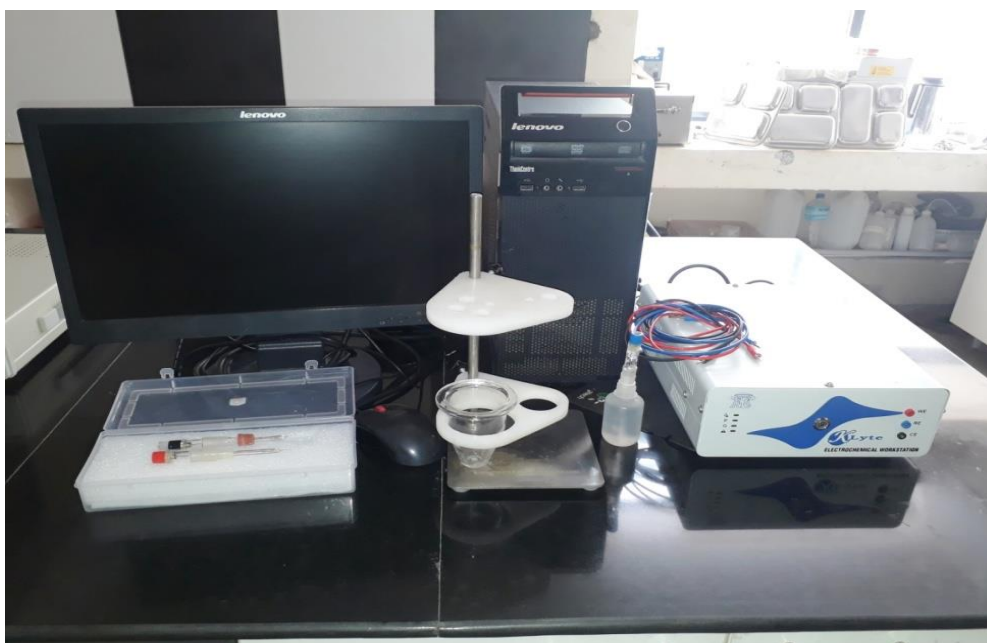
Potentiostat (Klyte 1.2) with customized software
