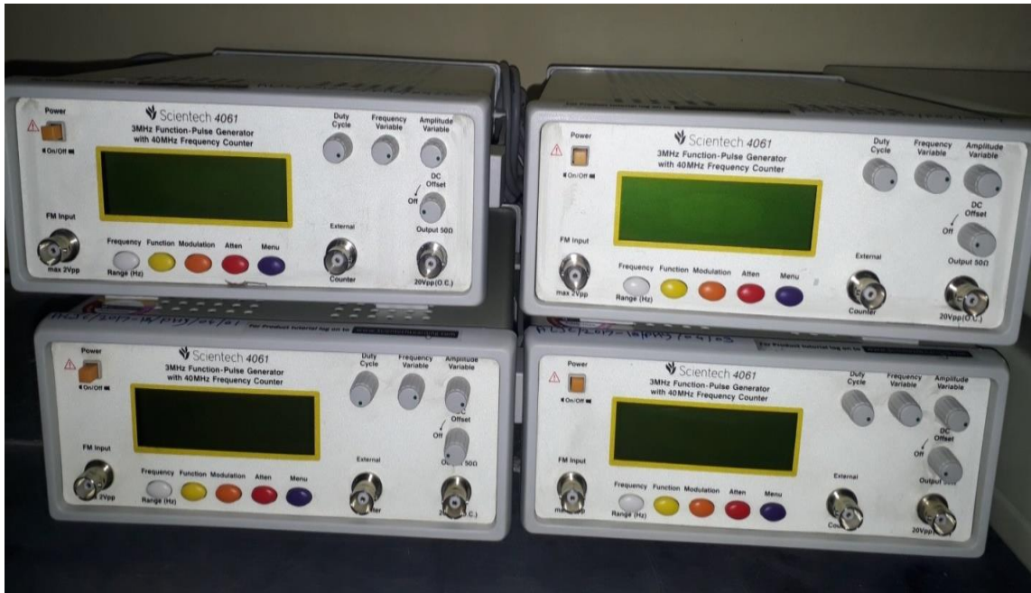
Function generator with 40MHz frequency
